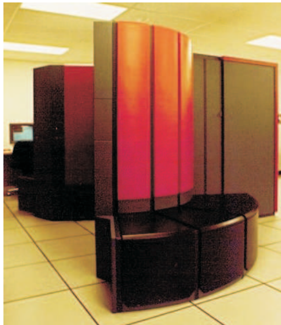
Figure 5.3: 1990: Cray Y-MP/432, a four-processor supercomputer with 256 MB of central memory.
