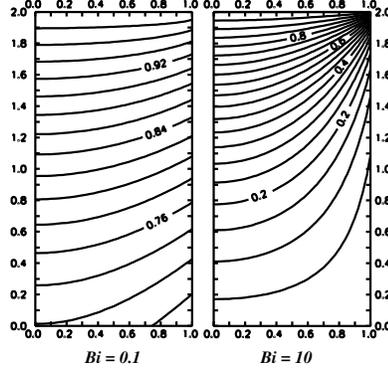
Figure 4.4: convective BC isotherms:  $Bi = 0.1$  (left),  $= 10$  (right)
