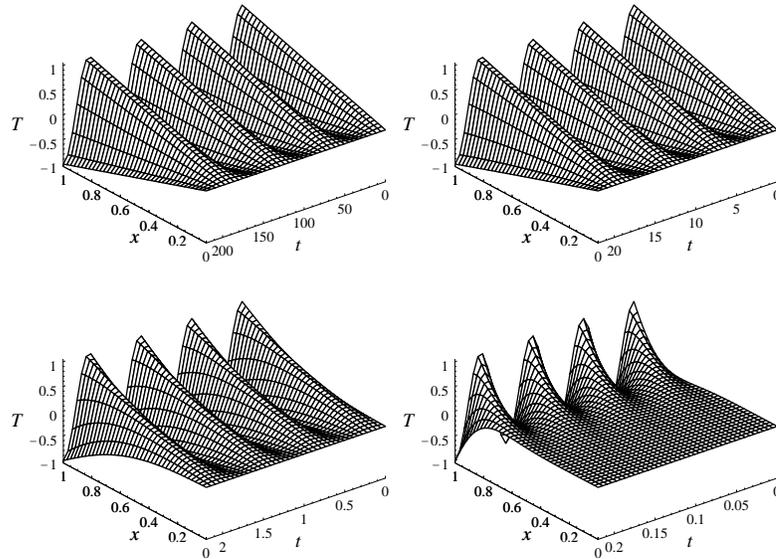
Figure 6.4: periodic surface temperature:  $\omega = 0.1$ (TL),  $1$ (TR),  $10$ (BL),  $100$ (BR)
