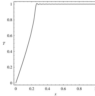
Figure 8.7: surface temperature distribution,  $a = 0.25$
