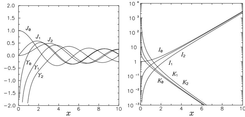
Figure 2.2: ordinary Bessel functions  $J_n$  and  $Y_n$ , and modified Bessel functions  $I_n$  and  $K_n$
