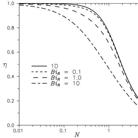
Figure 4.14: efficiency  $\eta$  for a circular pin fin
