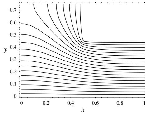
Figure 8.13: isotherms for the nonrectangular domain
