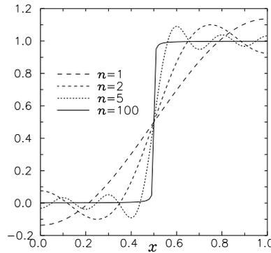
Figure 3.3: series representation of the step function
