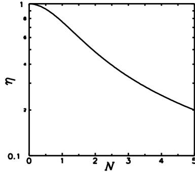
Figure 1.5: fin efficiency  $\eta$  for  $A_c = \text{constant}$
