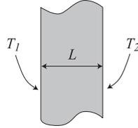
Figure 1.2: plane wall configuration
