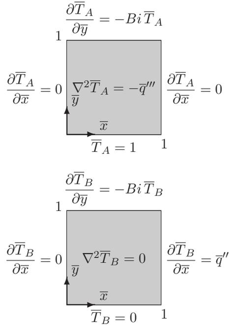
Figure 4.7: the two superimposed problems
