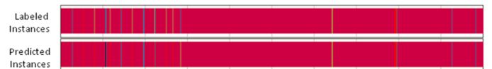
Figure 8 - Visualization of the labeled instances in time and the neural network prediction. Red are instances labeled and/or predicted as normal and other colors are instances labeled and/or predicted as other events (pump start, valve adjustment and/or batch changes).
