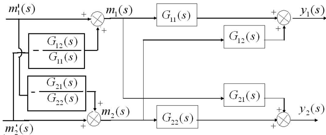
$$D_{21}(s) = -\frac{G_{21}(s)}{G_{22}(s)} \quad D_{12}(s) = -\frac{G_{12}(s)}{G_{11}(s)} \quad \mathbf{D}(s) = \begin{pmatrix} 1 & D_{12}(s) \\ D_{21}(s) & 1 \end{pmatrix}$$
