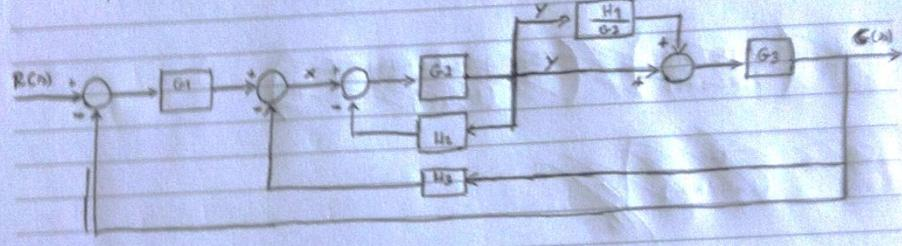
$$Y = G_2 [X - H_1 Y] \Rightarrow Y = G_2 X - G_2 H_1 Y \Rightarrow \frac{Y}{X} = \frac{G_2}{(1 + G_2 H_1)}$$
