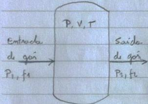
$$C_1 \cdot f_1(t) - C_2 \cdot f_2(t) = \frac{dm(t)}{dt}$$
