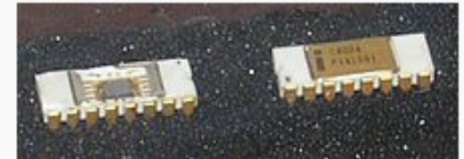
Intel C4004 microprocessor
